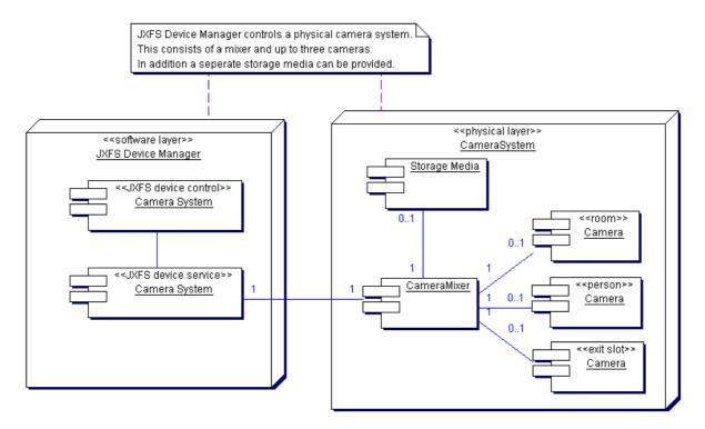
This configuration is the most common used in the field but can vary in different installations.
